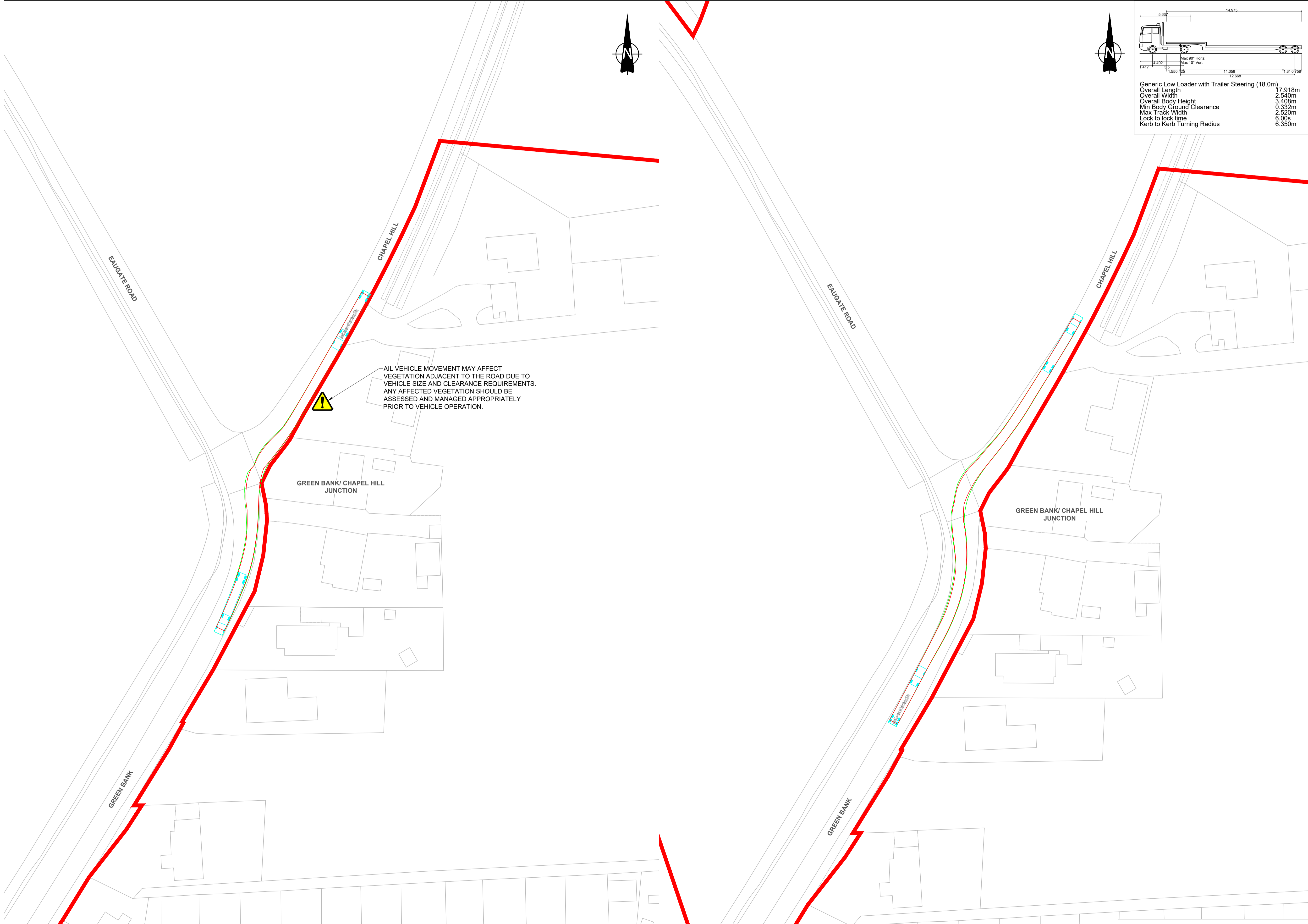
INSET A: 18m GENERIC LOW LOADER VEHICLE HEADING SOUTH-WEST ON CHAPEL HILL ROAD AND TURNING LEFT ONTO GREEN BANK ROAD - SCALE 1:500
